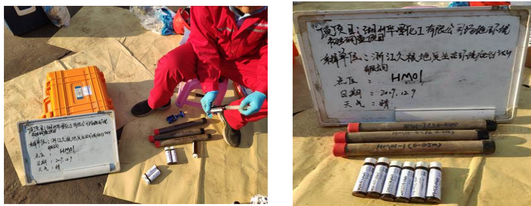
挥发性有机物非扰动土壤采样器装样
